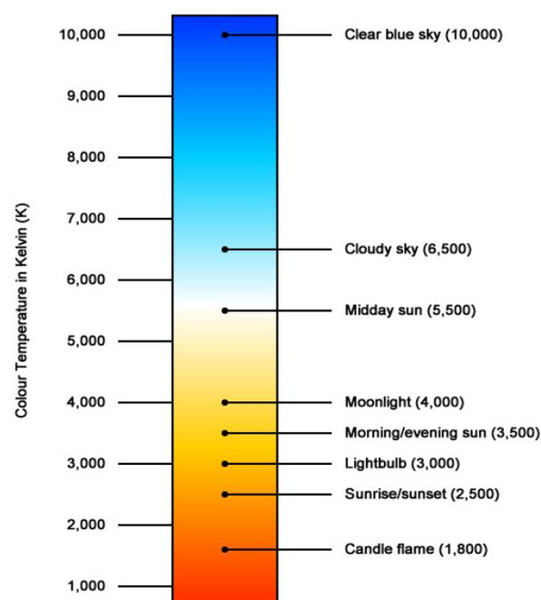
Generally LED lights are manufactured in the range 2400K to 6500K. Different colour temperatures are achieved by altering the makeup of the LED diodes used. This flexibility has provided the poultry industry with the ability to fine tune our choice of lights according to the needs of our birds.
