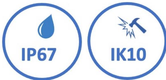
Firstly, there is the IP (Ingress Protection) Rating which is used to classify the different levels of sealing effectiveness provided by an electrical enclosure against foreign bodies such as water, dirt, ammonia gas etc.
