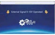
Pressing the "External Control" button enables connecting 0-10V signal for extenal control. Green indicator ON.
