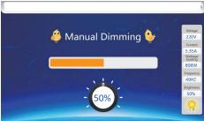
Pressing "Manual Dimming" enter the dimmer into "Manual Dimming"mode.
